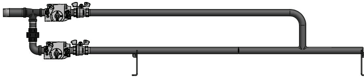
Figure 7-4_Gas Train 500,000 Btu/hr Model
